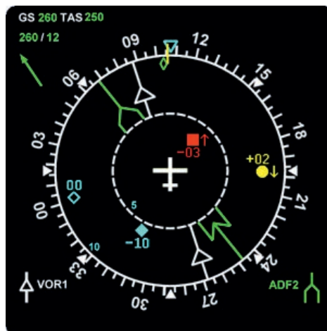
Figure 10: TCAS traffic display example – Electronic Flight Instrument System (EFIS).
