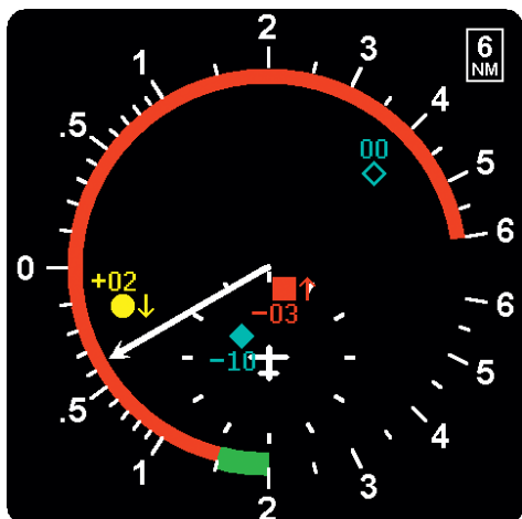
Figure 9: TCAS traffic display example – IVSI combined with TCAS traffic display.
