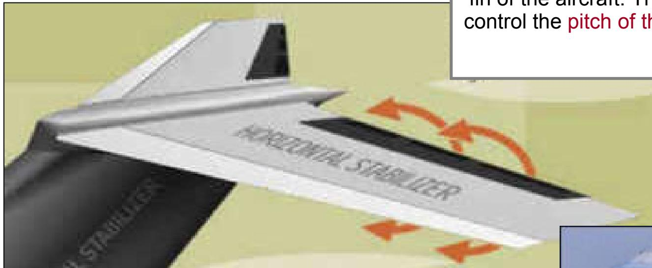
The stabilizer of the MD-83 has small pivoting wings and is mounted on the top of the vertical tail fin of the aircraft. The **horizontal stabilizers** help control the **pitch of the plane's nose** during flight.
