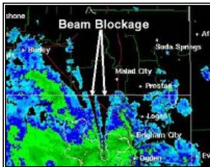
Figure 3-21. WSR-88D Weather Radar Beam Blockage on Base Reflectivity Product Example
