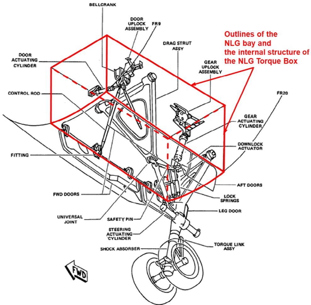
Fig. 5: Nose landing gear including landing gear well Source: Aircraft manufacturer, adaptation BFU
