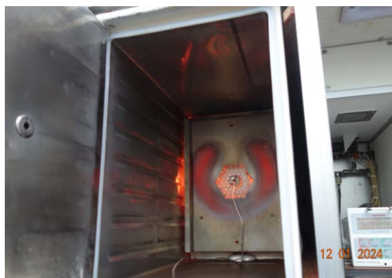
▲ Figure 5: The values measured by the various temperature meters on the test oven while duplicating an overheat condition. (Source: B/E Aerospace)
