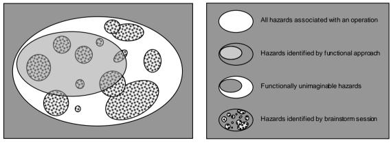
Figure 2: Functional and brainstorming approaches yield different hazard subsets
