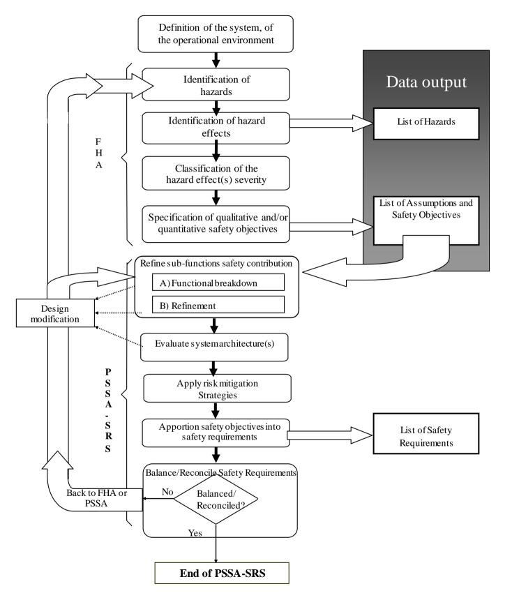
Figure 3.1: Safety Requirements Specification Process
