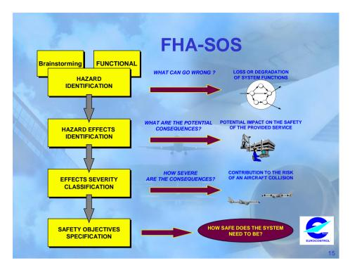
Figure 3.1: Safety Objective Specification (without "assess intended aggregated risk")
