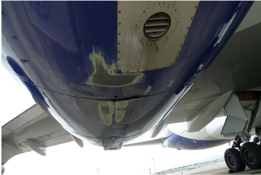
Photo 1: Damage at the Underside of No.3 Engine
