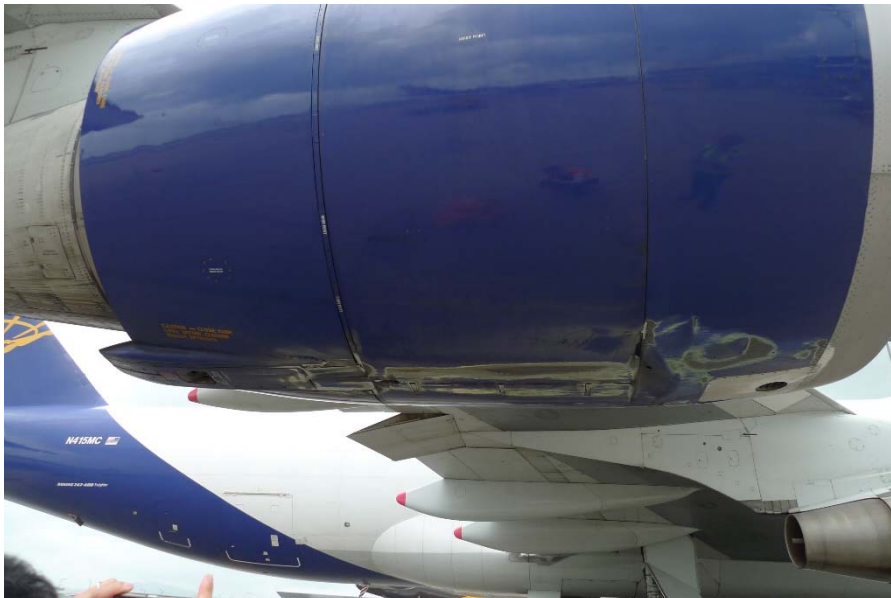
Photo 2: Damage at the Underside of No.4 Engine
