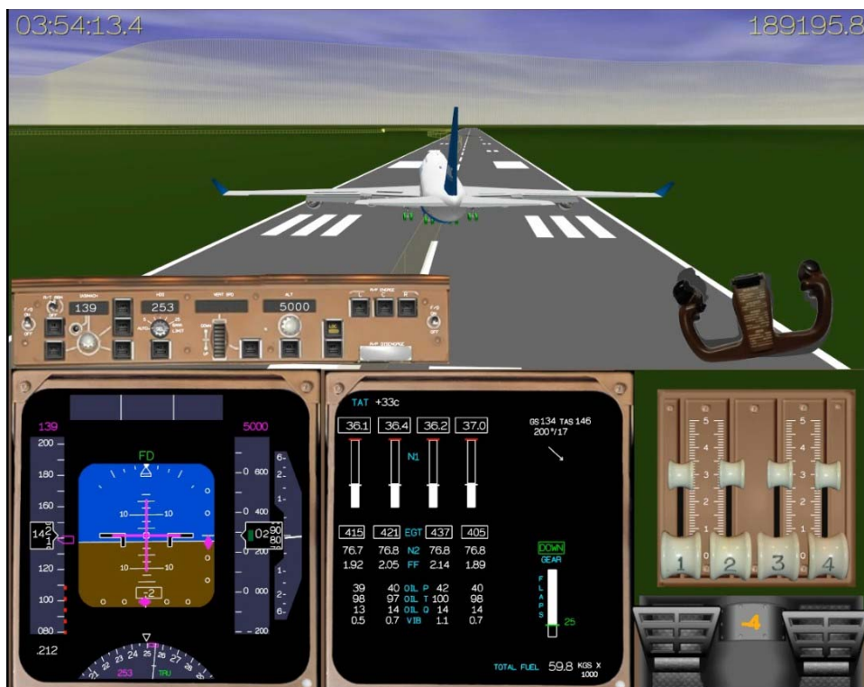
Figure 1: Aircraft in a Crab at Touchdown
