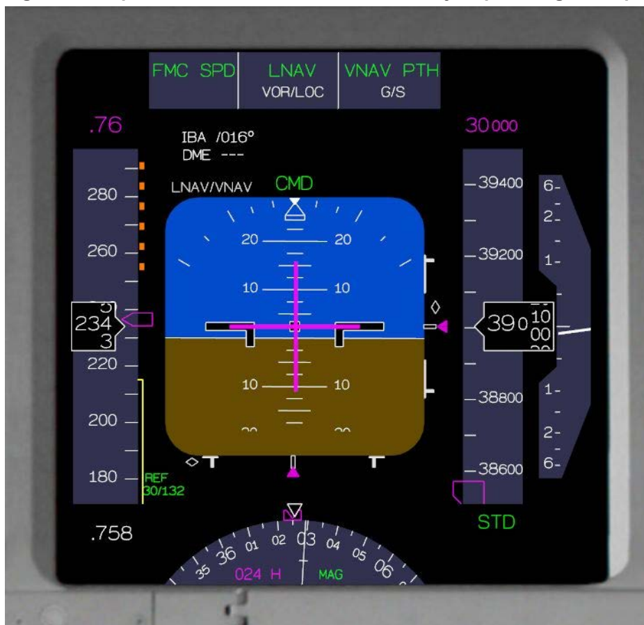
Figure 4 – Representation of the PFD at 2110:00 – just prior to glideslope capture
