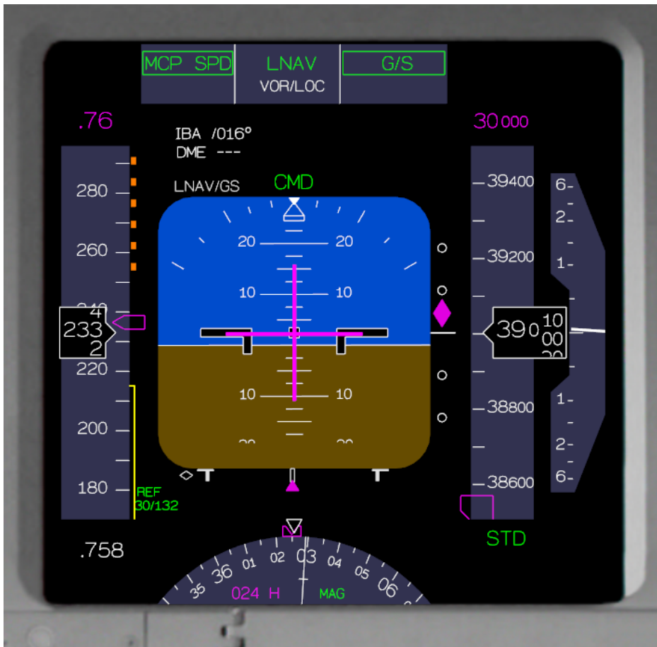
Figure 5 – Representation of the PFD at 2110:01 – glideslope capture
