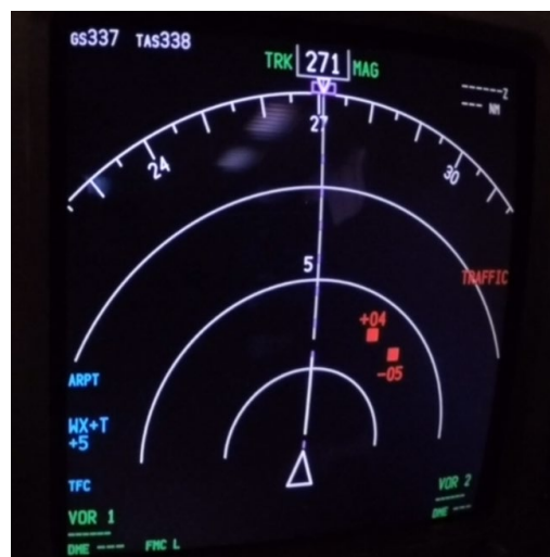
Figure 17: Actual traffic display implementation on Boeing 737-800.
