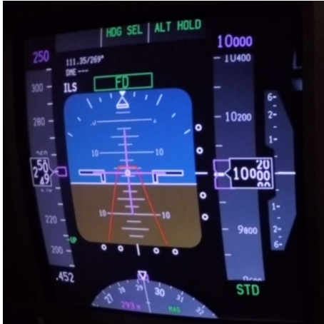
Figure 22: PFD with pitch cue display indicating a Climb RA on a Boeing 737-800.
