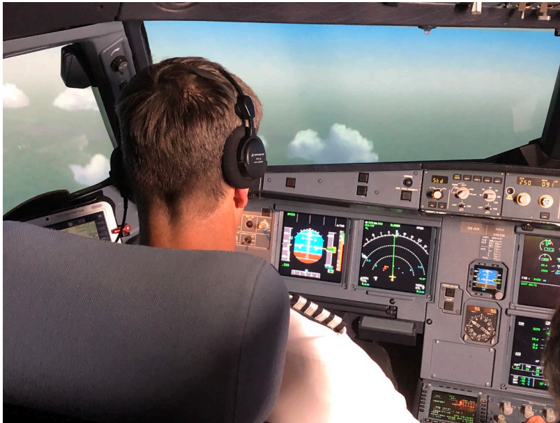
Figure 24: Primary Flight Display (left) and Navigation Display positions on Airbus A320.
