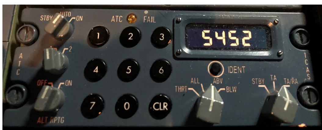
Figure 12: Example of TCAS/transponder panel on an Airbus A320.
