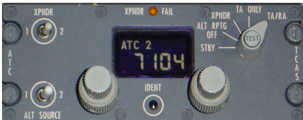
Figure 11: Example of TCAS/transponder panel on a Boeing 737-700.
