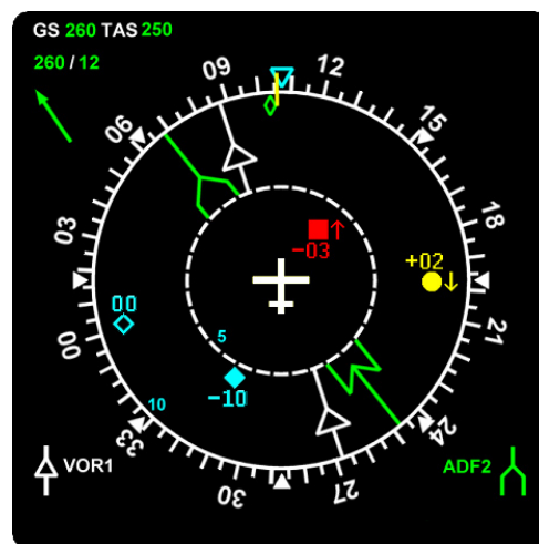
Figure 15: Traffic display example – Electronic Flight Instrument System (EFIS).
