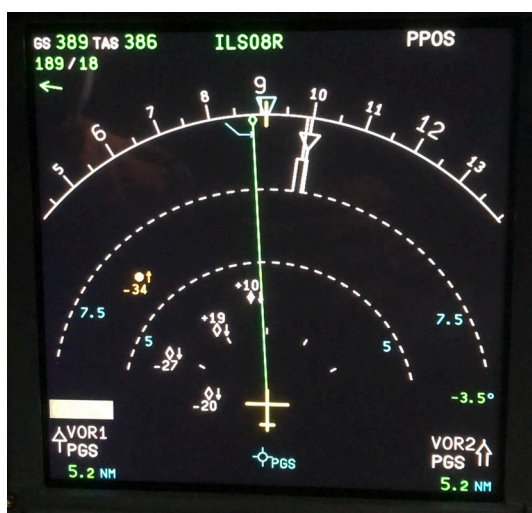
Figure 16: Actual traffic display implementation on Airbus A320.
