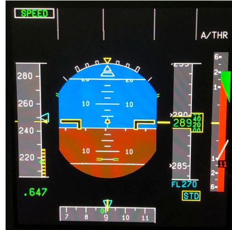
Figure 23: PFD with vertical speed tape indicating a Climb RA on an Airbus A320.
