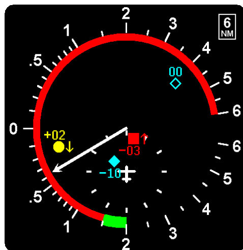
Figure 14: Traffic display example – IVSI combined with traffic display.
