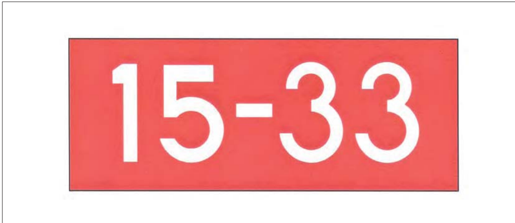
FIG 2-3-24 Runway Holding Position Sign
