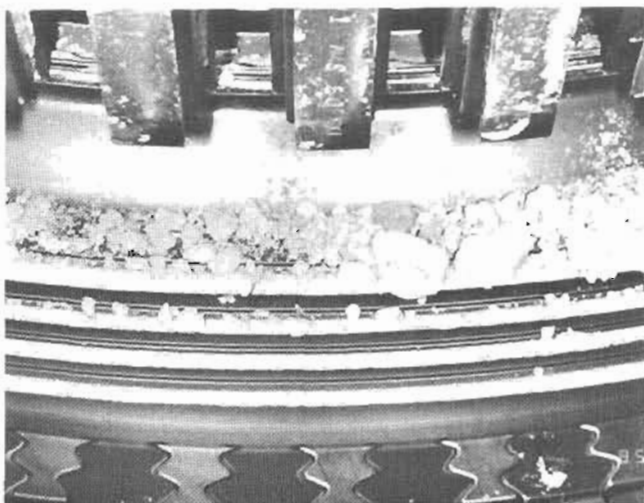
Figure 6. Accumulation of unmelted volcanic ash in the high-pressure-turbine rotor.
