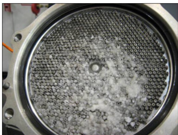
Ice accumulation on the inlet face of a Rolls-Royce RB211 Trent 800 Series Fuel/Oil Heat Exchanger during testing - Larger photo at: http://www.ntsbt.gov/Pressrel/2009/FOHEface.jpg
