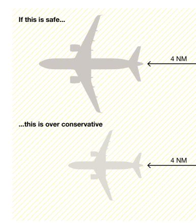
RECAT 1 FAA: The FAA decided to reclassify the aircraft by MTOW and wingspan. The RECAT FAA is implemented on several US airports.
