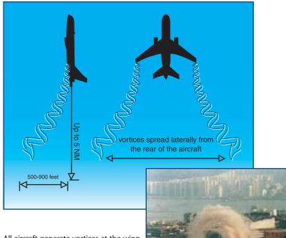
All aircraft generate vortices at the wing tips as a consequence of producing lift. The heavier the aircraft and the slower it is flying, the stronger the vortex.
