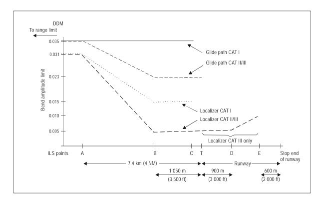
Figure C-1. Localizer course and glide path bend amplitude limits
